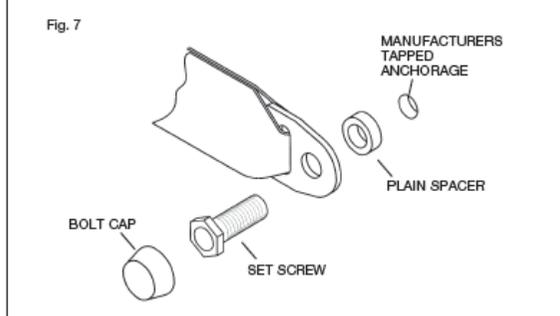
**2 POINT STATIC LAP BELTS WITH SNAP HOOKS**
